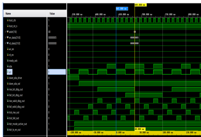
Figure 5. Functional Simulation Waveform of the HDR-DDR Enabled I3C Master Controller.
